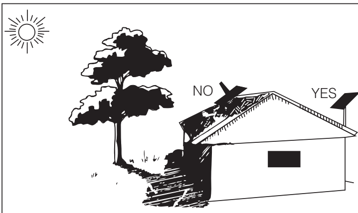
Figure 9.5 Module mounting site
