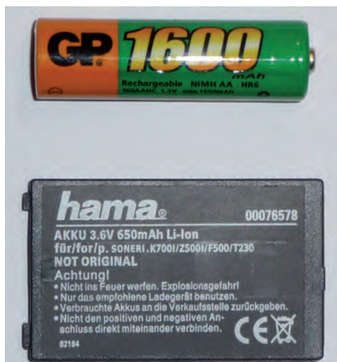
Figure 4.2 Rechargeable lithium ion and nickel metal hydride battery cells
