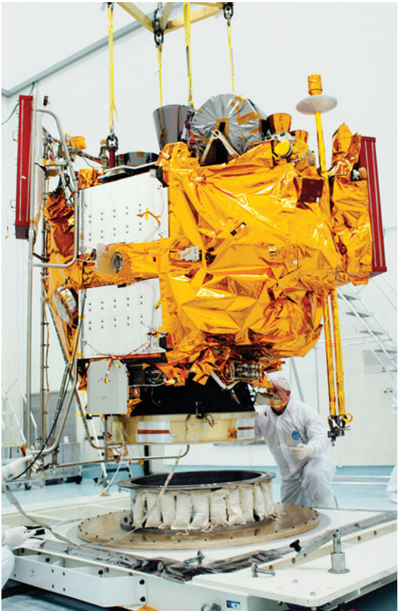
NASA technicians carefully lift the Messenger spacecraft in order to move it to a prelaunch testing stand. It was launched on Aug. 3, 2004.
