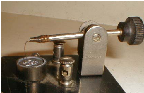
Figure 43.2: A galena crystal with cat's whisker. (©GNU-FDL,Wikimedia Commons.)
