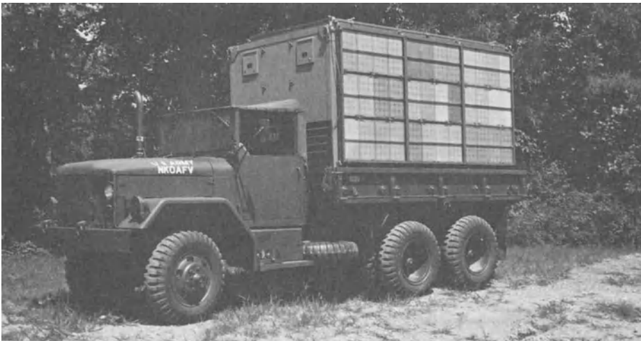
Fig. 1-6. Solar powered mobile communications station, deployed and stowed. (Courtesy of the U.S. Army Mobility Equipment Research and Development Command, Fort Belvoir, Virginia)
