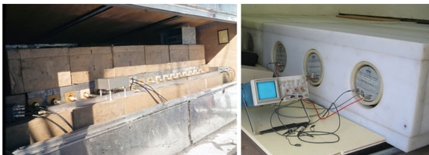
Fig. 6.1 18-IGY neutron monitor Jungfraujoch, Switzerland, ( left ) and 6-NM64 neutron monitor Athens, Greece ( right ). The digits 18 respectively 6 give the number of the counter tubes of the corresponding neutron monitor station
