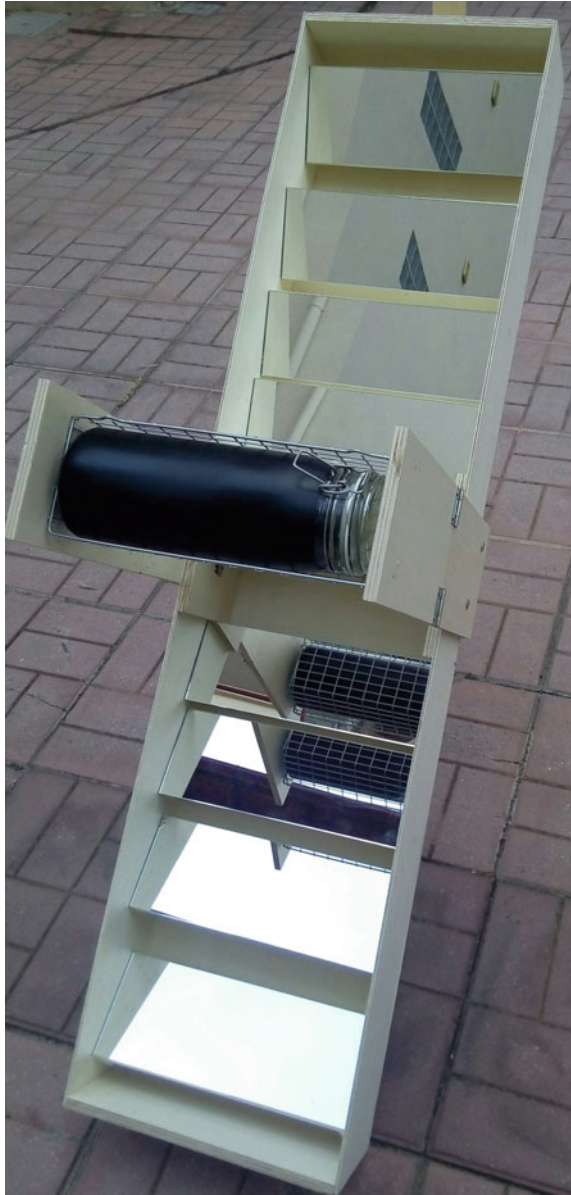
Fig. 8.11 Photograph of the complete Linear Fresnel Reflector Solar Cooker designed and developed in this chapter. It consists of the primary reflectors field, the receiver (the cooking vessel) and the supporting System
