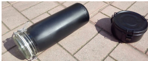
Fig. 8.4 Receivers (cooking vessels) used in the Solar Cooker developed in this chapter. Both of them are cylinder, but the first a is placed horizontally, while the second b is placed vertically, and they are used in the Linear and the Conical Fresnel Reflector Solar Cooker, respectively
