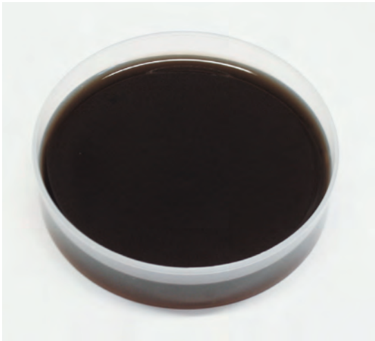
Figure 4.55 Damaged propylene glycol
