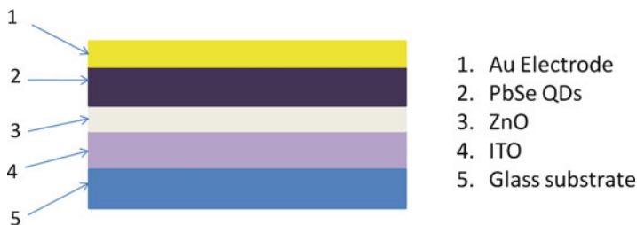
Fig. 9.6 Schematic of the PbSe QD sensitized bulk heterojunction device used to demonstrate MEG in a solar cell [43] consisting of: (1) A thermally deposited Au electrode; (2) 50–250 nm layer of PbSe QDs deposited in a layer by layer method with hydrazine and 1,2-ethanedithiol; (3) 40–50 nm of ZnO deposited on (4); and (5) ITO coated glass
