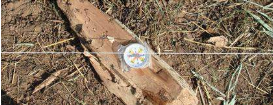
Determining and marking the north-south direction with the help of a compass
