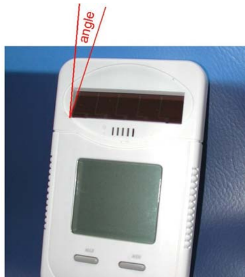
Fig. 7.21 Example of a wall-mounted sensor mounted so as to face the direction of the incoming light. (with permission [Randall-2005b])
