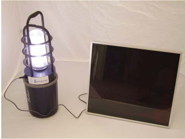
Fig. 7.15 Portable solar lamp (7 W compact fluorescent tube) with Solarex 12 V/5 Wp module and lead acid battery (12V; 3.4 Ah) (Credit Muntwyler Energietechnik AG).
