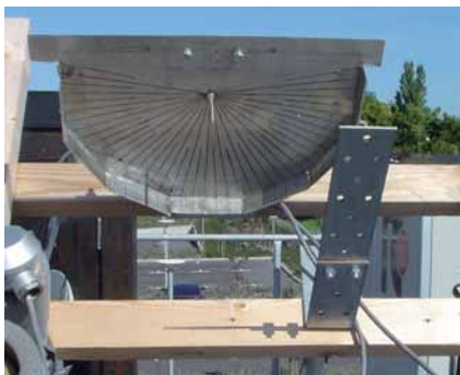
Figure 3.5 The device for measuring the transverse incidence angle on the glazing of the collector.
