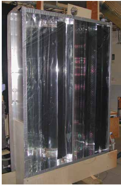
Figure 6.5 The roof MaReCo mounted in front of the solar simulator, with the absorbers placed vertically.
