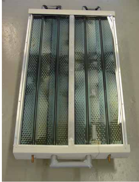
Figure 5.2 Collector A has standard Sun-strip absorbers of 143 mm.
