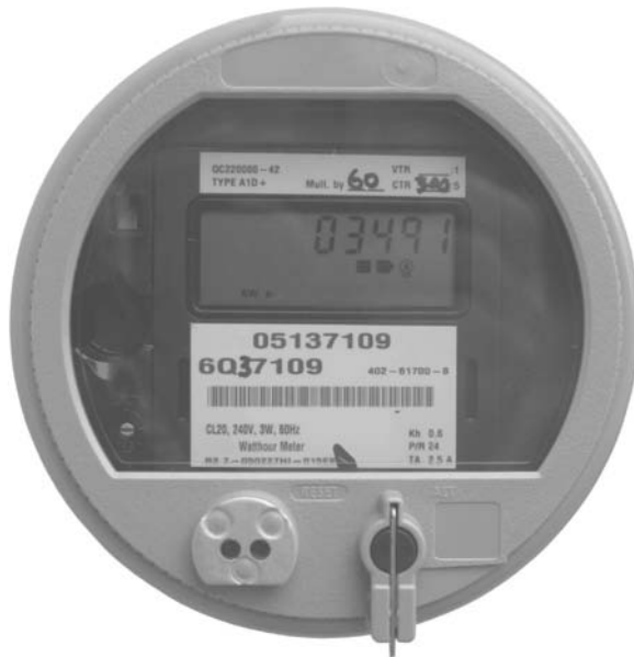
FIGURE 11.3 New Solid-State Digital Electric Meter Photo credit: Norman Morin.
