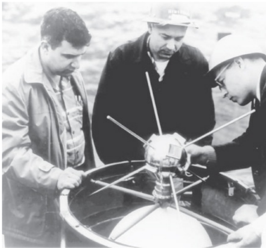
Solar panels with a purpose: GPS pioneer Roger L Easton (left) inspects the Vanguard 1 satellite with its six silicon solar panels.
