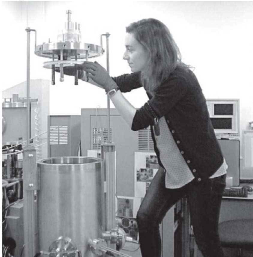
Nina Klein working on her self-built vacuum deposition chamber
