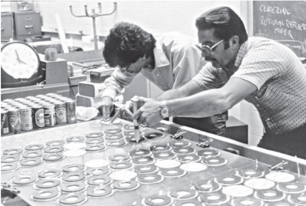
How to make a solar panel in 1981. Chris Case is on the left. The beer cans were just the right size and weight to hold the cells in place.
