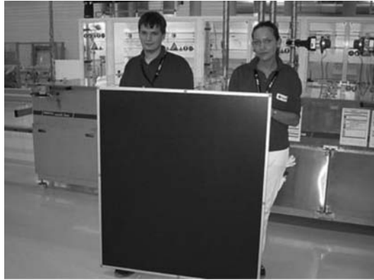
Figure 6.24 CSG module produced by CSG Solar, Germany (Source: USNW Annual Report 2009, reproduced with permission of Prof. Martin Green)
