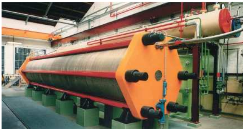
Figure 8: Norsk Hydro Alkaline electrolyser, which uses hydro-electricity to produce hydrogen
