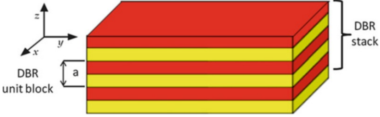
Fig. 2 Schematic of a one-dimensional photonic crystal (“distributed Bragg reflector,” DBR). The DBR consists of several DBR unit blocks. Each DBR unit block consists of alternating layers of two materials with different dielectric constants, with a period a (From Ref. [37])
