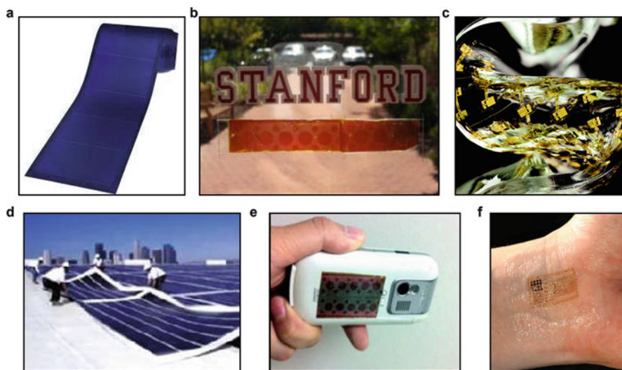
Fig. 3 (a) Photograph of flexible a-Si solar cells deposited onto stainless steel substrates, prepared by roll-to-roll process [19]. (b) Optical image of a flexible Si solar cell printed on a glass window surface [20]. (c) Optical image of c-Si photodiode arrays printed onto PDMS substrates [17]. (d) Photograph of flexible a-Si solar modules for building integration [19]. (e) Flexible solar cells mounted on a portable device [20]. (f) Optical image of epidermal electronic circuits (Reproduced with permission. Copyright 2008 Wiley-VCH. Copyright 2012 Nature Publishing Group. Copyright 2008 PNAS)
